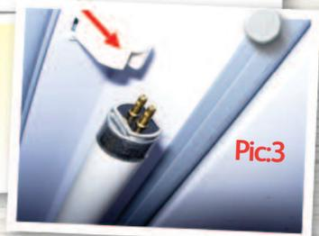
To fit the new tube simply push it into both the left and right connector slots at the same time, taking care that the pins slide up as in reverse of **Pic:3**.
